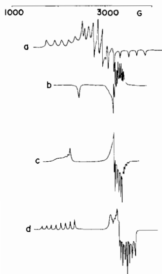
Figure 3. ESR spectra of cobalt(II) complexes obtained at 77 K: a) [Co(14-b)] + , b) [Co(14-c)], c) [Co(15-c)], d) [Co(16-c)].
